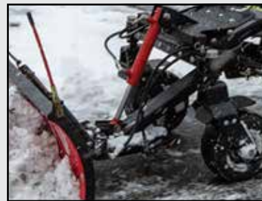
SNOW PLOW MOUNT SYSTEM Hydraulic lift, pitch, & down pressure
